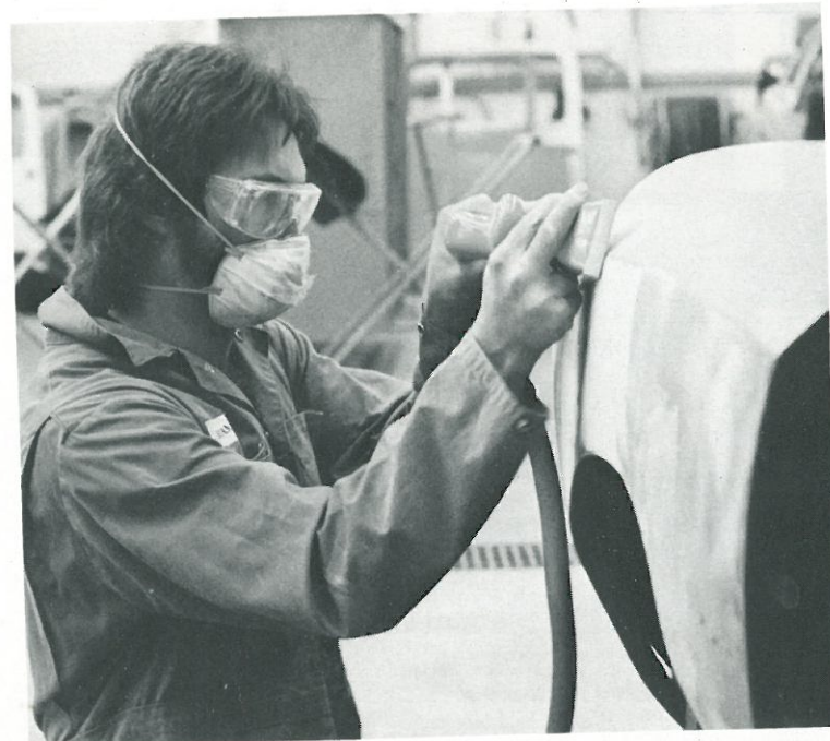
Above Left: Brian Jewett, second year Autobody Mechanic, levels body fill on an inhouse project, the restoration of a '77 Monte Carlo. Above Right: Barry Martyn, a third year welder, bevels a 4" pipe to prepare for T.A.W. Gas tungsten Arc Welding, commonly known as T.I.G.
